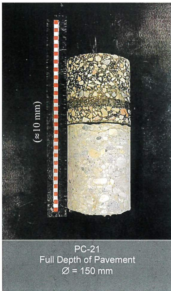
Photograph 21: Specimen from Sargent Avenue, Eastbound Median Lane
