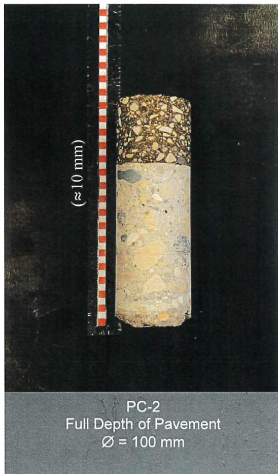
Photograph 2: Specimen from Ellice Avenue, Eastbound Median Lane
