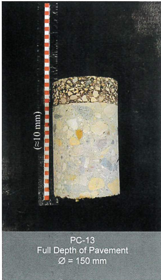
Photograph 13: Specimen from Sargent Avenue, Eastbound Median Lane
